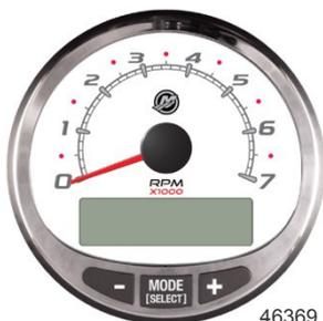
1. Press the "MODE/SELECT" and "+" buttons simultaneously for approximately two seconds or until the "MENU" screen appears.
