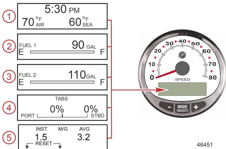
When the ignition is turned on, the speedometer will show the last screen that was displayed before the ignition was turned off.
