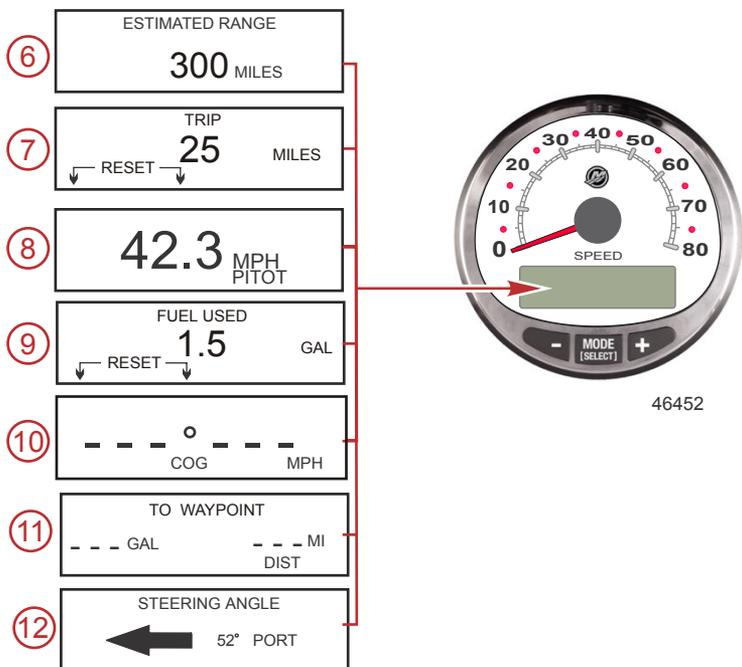
6. **Estimated Range:** The estimated range is based on boat speed, fuel consumption, and fuel remaining in the tank. The numbers displayed are an estimate of the distance you can travel with the remaining fuel. Speed input required (paddle wheel, pitot pressure, or GPS).
