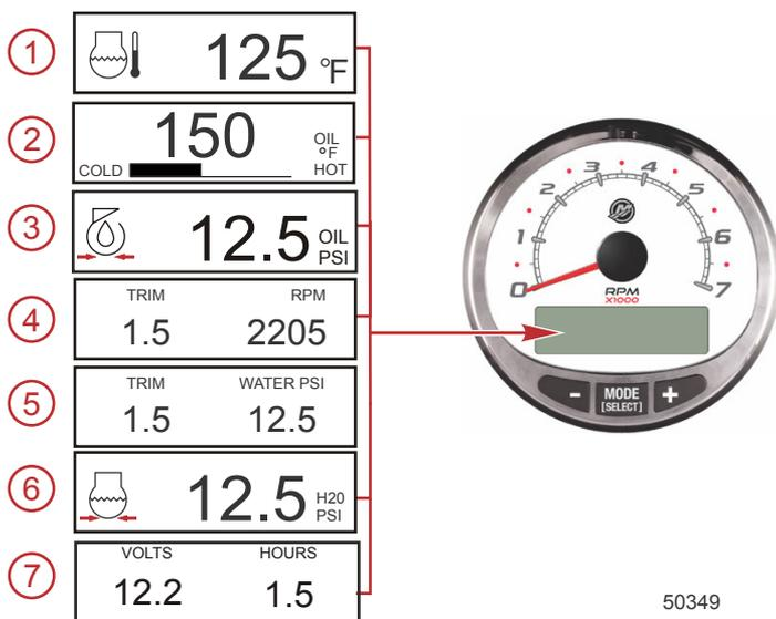
1. **Temperature:** Displays the engine coolant temperature.
