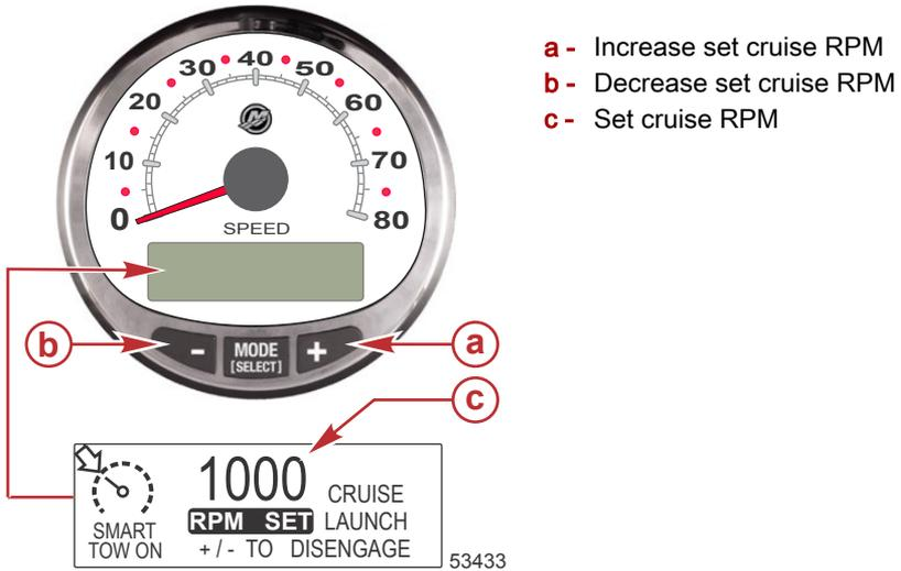
**NOTE:** The cruise control minimum maximum range may change depending on engine model.
