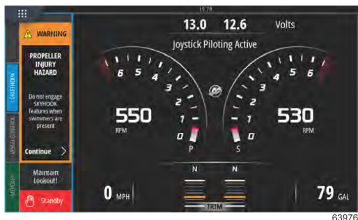
Propeller injury hazard warning
