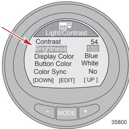
4. Press the MODE button to save the brightness setting.
