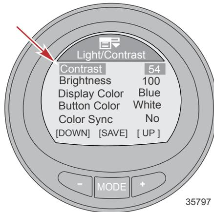
3. Press the MODE button to save the contrast setting.
