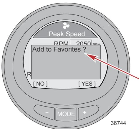
5. Press the "+" button to save the screen to the Favorites menu. If the screen is not wanted, press the "-" button to discard the screen option.
