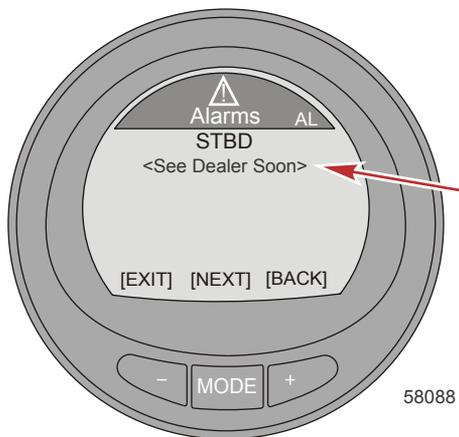
6. Press the MODE button to view the next fault text, if available.
