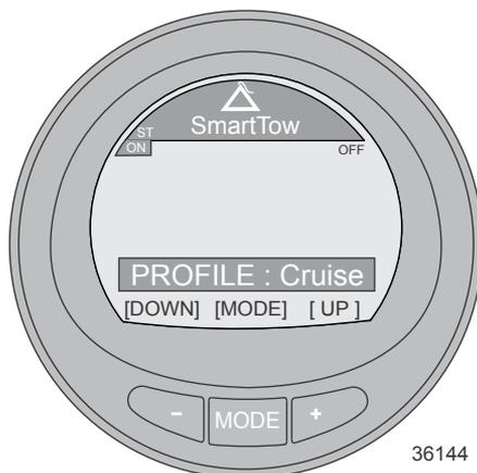
2. Press the "-" or "+" button when the profile screen is visible to advance through or change the launch modes, and all of the customized launch settings.
