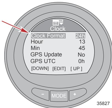
6. Use the "+" or "-" button to highlight the options and use the MODE button to turn the option on—Yes, or off—No.
