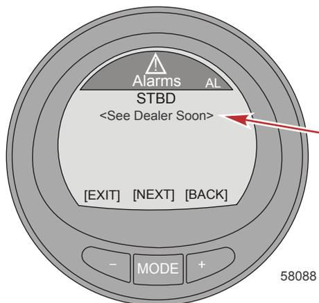
4. Press the "+" button to go back to the component identification or press the "MODE" button to view the next alarm.
