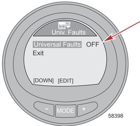
6. Press the "-" button to highlight the Exit option and press MODE to exit the Universal Faults menu.
