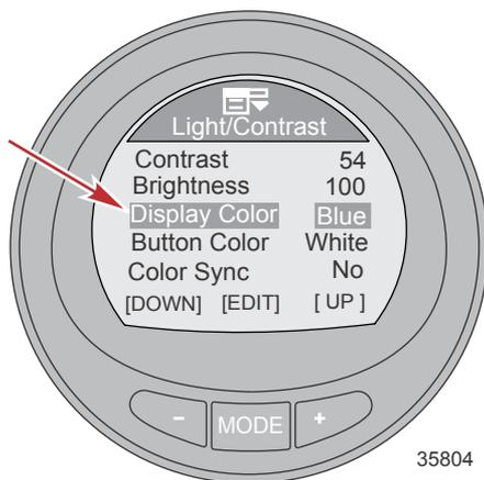
4. Press the MODE button to save the display color setting.
