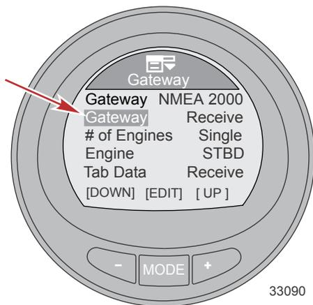
8. Press the "-" button to highlight the # of Engines menu.
