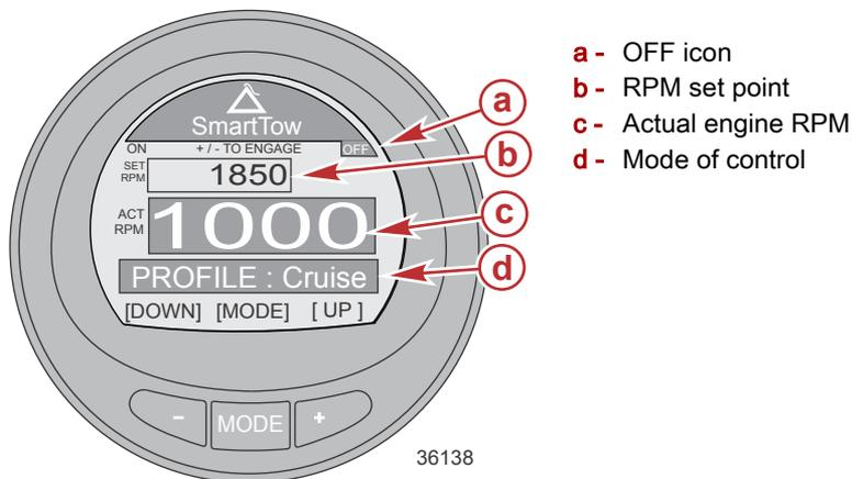
1. To engage the Smart Tow function, press the "-" and "+" buttons at the same time. The Smart Tow ON icon will be highlighted in the upper left corner and the information above the SET RPM window will be changed to +/- TO DISENGAGE. When Smart Tow is engaged, the ON icon will remain on and be visible on all of the monitor screens.
