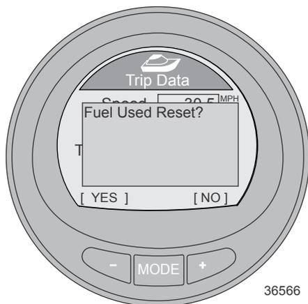
8. Press the "-" button to return to the Main Menu, or press the MODE button to go to the next screen.
