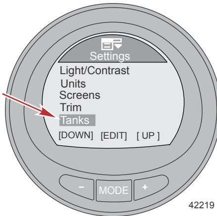
5. Press the MODE button to edit the Tank 1 Type option.
