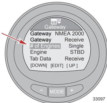
10. Press the "-" button to highlight the Engine menu.
