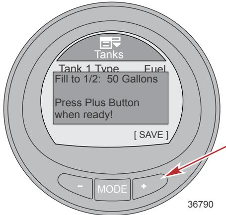
21. Add 25 percent more fuel capacity to the fuel tank. Press the "+" button to save the calibration.
