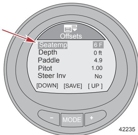
7. Use the "+" or "-" button to highlight the options and use the MODE button to turn the option on—Yes, or off—No.
