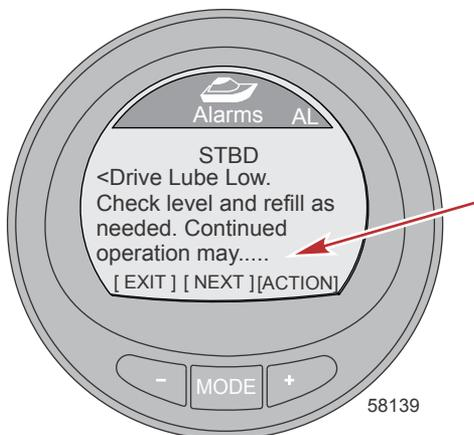
8. Press the "+" button to view the remaining long descriptive text.
