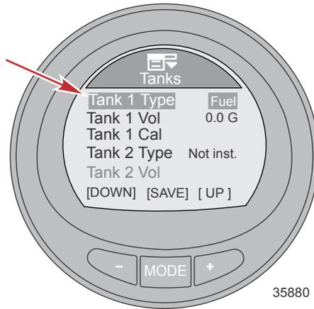
7. Press the MODE button to exit the Tank 1 Type option.
