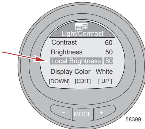
4. Press the MODE button to save the local brightness setting.
