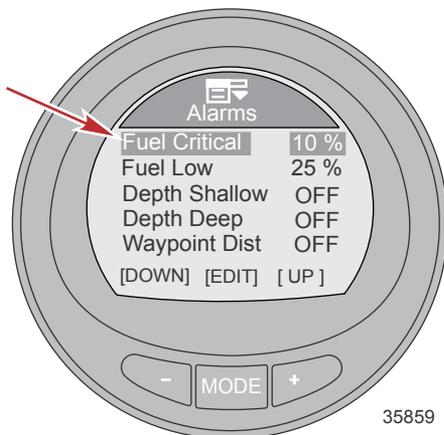
7. Press the MODE button to exit the Fuel Critical option.
