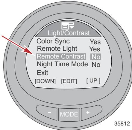
3. To exit the Light/Contrast menu, press the "-" or "+" button to highlight the Exit option. Press the MODE button to exit the Light/Contrast menu.
