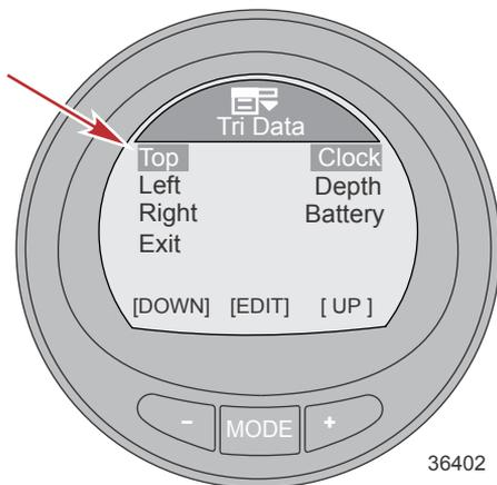
6. Press the MODE button to exit the Top screen data option.
