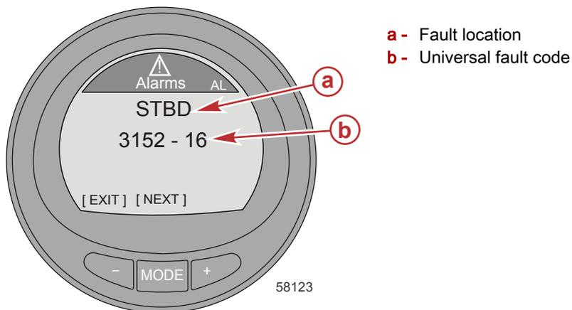
If a problem can cause immediate engine damage, the Engine Guardian System will respond to the problem by limiting engine power. Immediately reduce the throttle speed to idle and refer to the warning messages. If the "MODE" button is pressed to display a different screen, the flashing alarm signal "AL" will appear in the upper right corner to indicate there still is a problem. Refer to the appropriate service manual for further explanation of the problem and the correct action to take.
