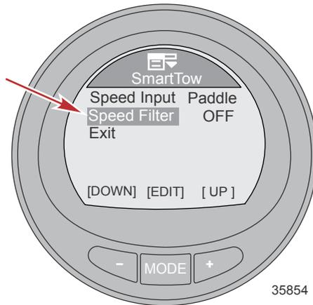
8. Press the "-" button to highlight the Exit option and press MODE to exit the Smart Tow menu.
