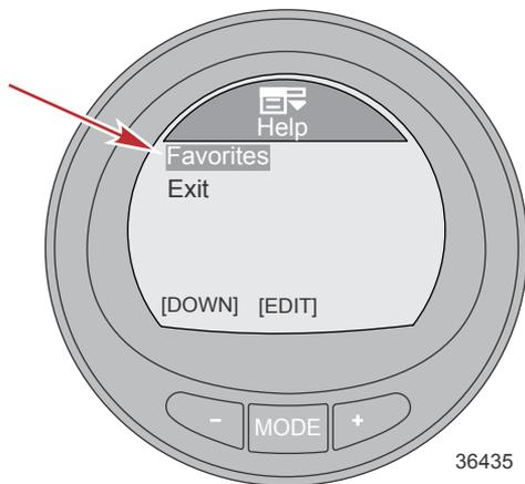
6. A window will pop-up stating to hold the "+" and "-" buttons down when the screen you desire to be part of the Favorites is visible on the monitor.
