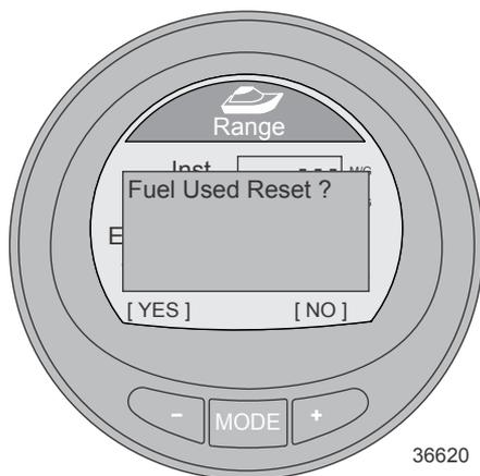
6. Press the "-" button to return to the Main Menu, or press the MODE button to go to the next screen.
