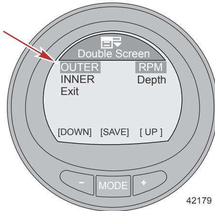
6. Press the MODE button to save the OUTER screen data option.
