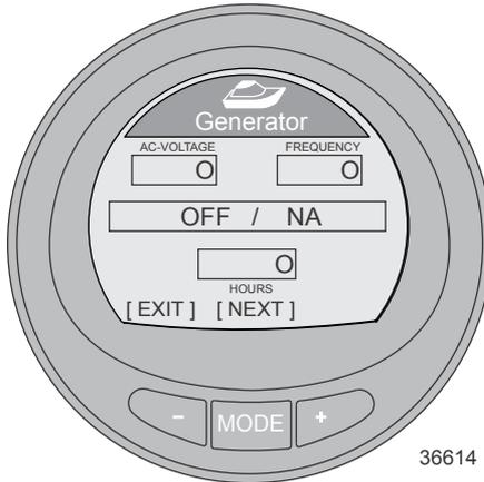
Press the "-" button to return to the Main Menu, or press the MODE button to go to the next screen.
