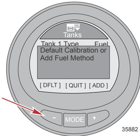
15. Press the MODE button to finish—OK, and exit the Tank 1 Cal option.
