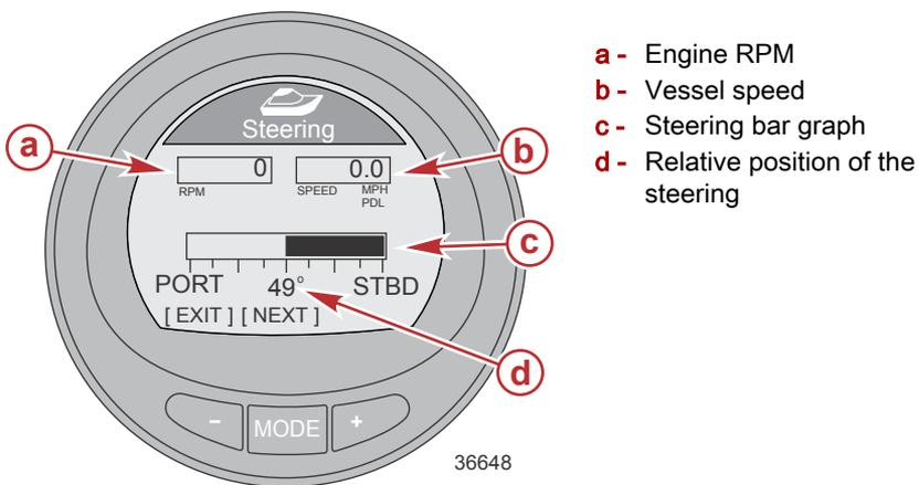
Press the "-" button to return to the Main Menu, or press the MODE button to go to the next screen.
