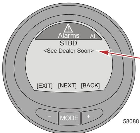
4. Press the "+" button to return to the short descriptive text fault screen, or press the MODE button to view the next alarm fault, or press the "-" button to exit the Alarms menu and return to the Main Menu.
