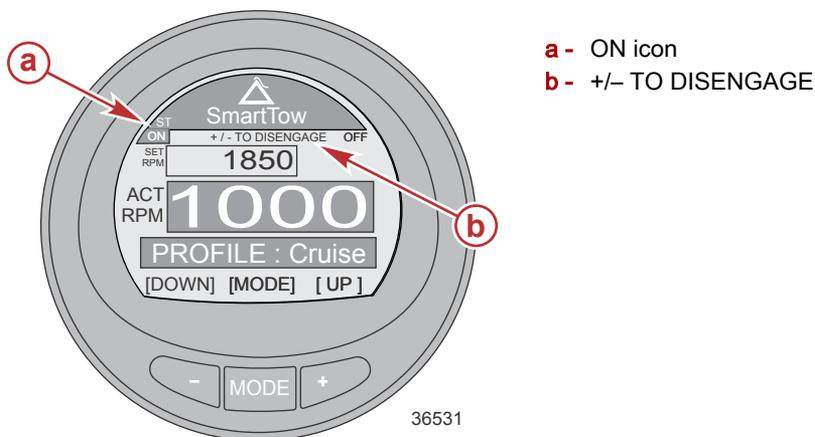
2. Shift the drive unit into forward gear. The throttle must be above the set cruise RPM or speed for the Smart Tow cruise to function. When the throttle is moved below the set cruise engine RPM or speed, the engine RPM will decrease with the throttle movement.
