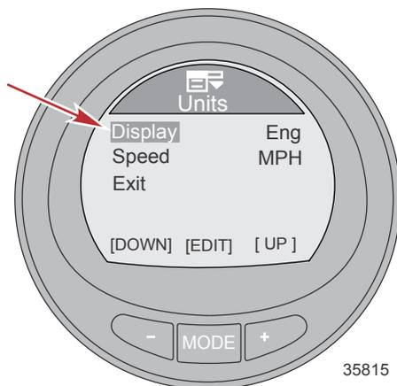
6. Press the "-" button to highlight the Speed unit.
