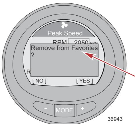
3. Press the "+" button to remove the screen from the Favorites menu. Press the "-" button to keep the screen as a favorite.
