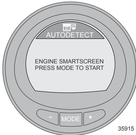
If the gauge shows a warning of "NO STARBOARD ENGINE" or "MULTIPLE STARBOARD ENGINES," the engine location (port and starboard) must be selected by an authorized dealer equipped with the computer diagnostic system (CDS) tool.
