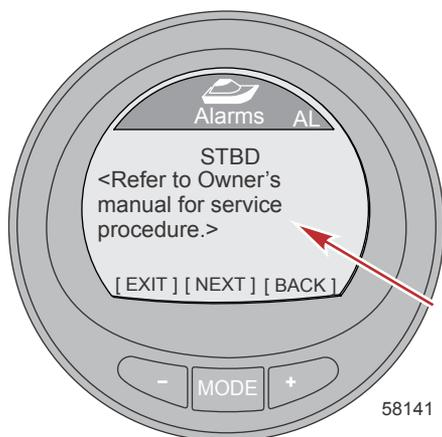
10. Press the "+" button to return to the short descriptive text fault screen, or press the MODE button to view the next alarm fault, or press the "-" button to exit the Alarms menu and return to the Main Menu.
