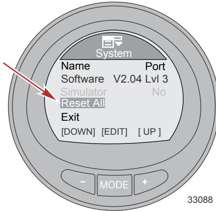
13. Press the "+" button to reset the gauge to the factory default settings or press the MODE button to quit the reset function. Press the "+" button to confirm the gauge has been reset to factory defaults.
