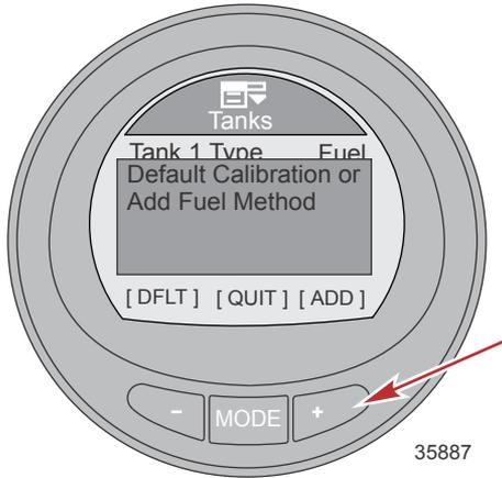
17. Press the "+" button to save and edit the Add Fuel Method of calibration.
