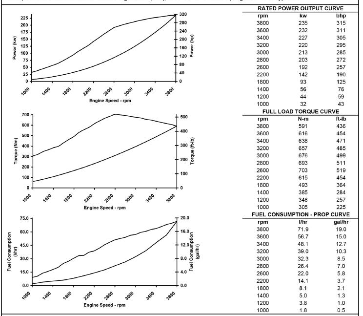
Rated Conditions: Ratings are based upon ISO 15550 reference conditions; air pressure of 100 kPa [29.612 in Hg], air temperature 25deg. C [77 deg. F] and 30% relative humidy. Power is in accordance with IMCI procedure. Member NMMA.
