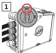
Verify the power switch on the Power Center, if equipped, is turned to the **OFF** position.
