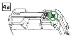
Charging a single 2.3 kWh battery is done through the charging port on the top of the battery.
