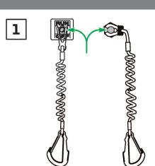
Engage the lanyard into the safety switch. Secure the clip end to the operator.
