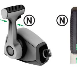
Depending on the control model of the outboard, verify the remote control or tiller is in the neutral position.
