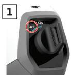
Remote model: To power off the outboard, turn the key to the **OFF** position.
