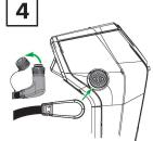
For tiller models, ensure the battery cable on the outboard is connected and locked. Fully engage the cable connector into the socket and twist-lock the connector collar fully.
