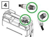
Install weather caps on the batteries and cables. Remove any clamping brackets or tie-downs and remove the batteries from the boat.
