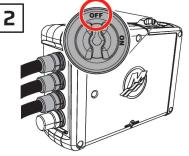
If the boat is equipped with more than one battery, verify the Power Center switch is turned to the **OFF** position.
