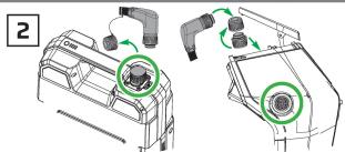
Remove all weather caps from the batteries, outboard, and power cables. Mate the battery weather cap to the tethered cap from the cable. For tiller models, mate the outboard weather cap to the power cable weather cap and stow them in the outboard by sliding the hood release. Verify charging ports on batteries and Power Center are closed.
