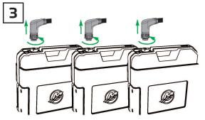
Disconnect the battery terminal connectors. Twist the connectors counterclockwise and lift up.
