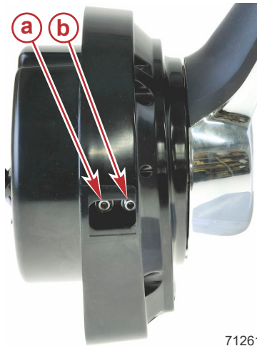
Panel mount ERC (ERC shown not installed, access cover removed)
