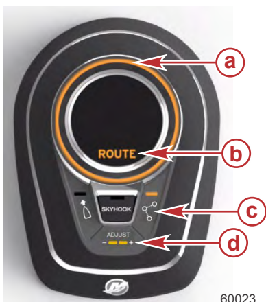
Top view of joystick, showing route mode engaged and approaching a waypoint
