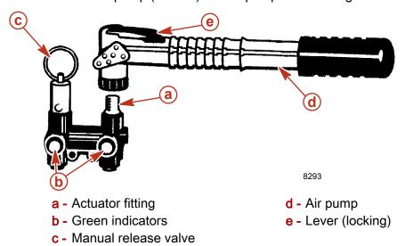
6. Pump air into the system until both green indicators extend and water drains from both sides of the engine. The port side will begin draining before the starboard side.
