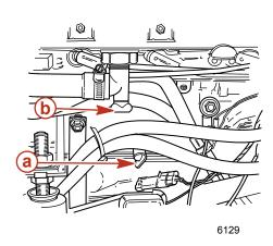
**b** - Bottom of exhaust manifolds
