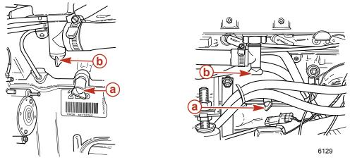
a - Cylinder block drain plug
