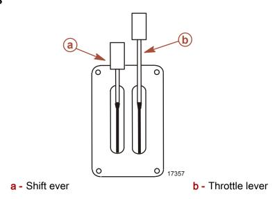
**Shift Lever -** Shift functions are controlled by the movement of the shift lever. Shift into reverse by moving the shift lever to its aft position. Shift into neutral by moving the shift lever to its center position. Shift into forward by moving the shift lever to its forward position.
