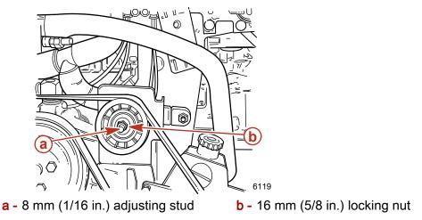
8. Operate the engine for a short period of time and recheck the belt adjustment.
