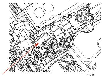
4. A 20 amp fuse may be located in the ignition switch "I" terminal lead to protect the electrical system. Check for blown fuse if the ignition key is turned to the "START" position and nothing happens (and circuit breaker is not tripped).
