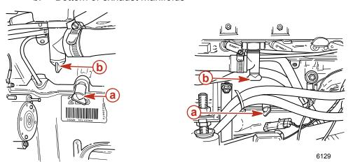
a - Cylinder block drain plug
