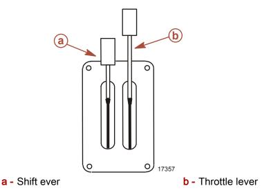
**Shift Lever -** Shift functions are controlled by the movement of the shift lever. Shift into reverse by moving the shift lever to its aft position. Shift into neutral by moving the shift lever to its center position. Shift into forward by moving the shift lever to its forward position.
