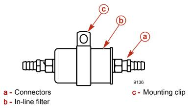
9. Install and torque screw and washer through the mounting clip into the stringer.
