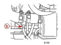
**b** - Fuel cooler to thermostat housing
