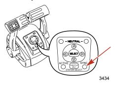
To disengage, move one or both control handles until they are more than 5° apart, reduce engine speed below 900 RPM, or increase engine speed beyond 95%.
