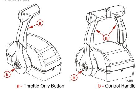
**Throttle Only Button -** Allows engine throttle advancement without shifting the engine. This is done by disengaging the shift mechanism from the control handle. The throttle only button can be depressed only when the remote control handle is in the neutral position.
