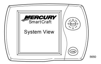
Your power package may be connected to the Mercury SC5000 SmartCraft System View display. The display monitors and reports information ranging from basic operating data to engine alarm data.
