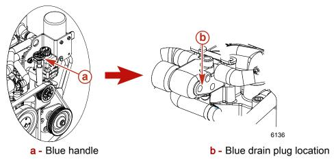
4. Visually verify that water is draining. If water does not drain, remove the blue drain plug from the distribution housing and drain manually.
