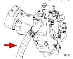
c. Using appropriate connector, connect the flushing water hose to the transmission seawater inlet fitting.
