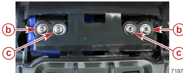
Dual-handle console ERC a - Access cover b - Detent adjustment screws c - Handle friction adjustment screws
